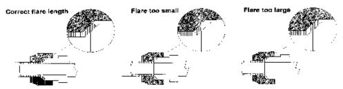
The proper flared tubing should resemble the diagram on the left (pictured above).
