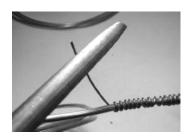
5. After the V notch has been filed into the capillary tube take a pair of pliers and bend the end of the capillary tube at the notch so the end of the capillary tube breaks off. Assure that the end of the tube is open to allow the refrigerant to flow through to the evaporator. The inside diameter of the capillary tube is very small (.022 inch).
