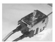
spade terminals to the tab on the thermostat (015-0282) marked "3" and the other female spade terminal to either of the two thermostat tabs marked "4". Run the wire along the same route as the copper tubing to the condensing unit. Attach two more female spade terminals (290-0001) to the stripped ends of the 18/2 wire. Attach these terminals to the Power Module "T" and "C" tabs. Tie the thermostat wiring to the refrigerant line set with cable ties (400-0911) every 18 inches.
