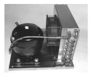
15. Flux the end of the discharge copper tubing and insert into the 3/16" copper union (025-0205) that is protruding from the top connection tube of the condenser (012-1001). Solder all the joints according to the preparation procedures mentioned previously in the Preparation Section.
