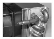
11. Place the 3/16" copper union (025-0205) into the 3/8" to 1/4" fitting reducing copper union (025-0301 from the previous step) at the top of the condenser (012-1001). This will be soldered in place once the
