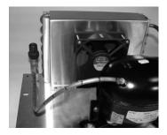
21. Mount the discharge base valve (096-0040) in the remaining square hole on the base plate (055-0104). Label the valve with "D" to identify as the discharge valve before mounting. The base of the valve has a square cutout on the bottom that fits in the square hole of the base plate and prevents the valve from turning on the base. Position the valve so
