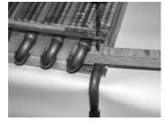
Damaging the condenser tubing will make the condenser unusable. <u>Damage of this sort is not warranted in any way by RParts</u>. A new condenser must be purchased before kit building continues.
