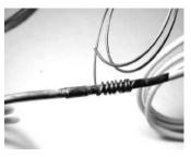
4. Now take the corner edge of a small fine triangular file and file a notch part way through the capillary tube on both sides. File this notch within an inch or two of the end of the capillary tube as shortening the capillary tube too much will affect the performance of the unit. The capillary tube is what regulates the amount of refrigerant entering the evaporator.
