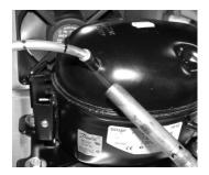
20. After the solder connection has cooled, gently bend the attached 1/4" copper tubing to route it in place to mate it with the male flare fitting on the suction base valve (096-0040) as shown in the photo. Make large diameter bends and avoid kinking the tubing. Tighten the flare nut firmly to the suction base valve with two wrenches.
