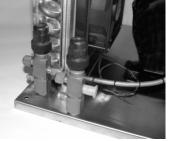
the two flare fittings are pointing as shown. Attach the valve using the hex head mounting bolt (400-0010), lock washer (400-0012), and flat washer (400-0011) to hold it in place from underneath the base plate. Tighten firmly using an appropriately sized wrench.
