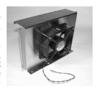
5. Place the fan shroud (055-0181) over the condenser (012-1001). The circular opening of the fan shroud should be on the compressor side with the top of the shroud slipping over the top of the condenser. Line up the two holes in the bottom mounting flange of the fan shroud with the two holes in the base plate (055-0104) and attach with two 1/2" Phillips
