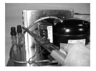
the wire tool to crimp each connection. Twist the fan wires together. The red wire terminal attaches to the small "+" connection on the compressor power module, and the black wire terminal attaches to the "F" connection on the power module. Push the terminals firmly onto the appropriate connections on the module.
