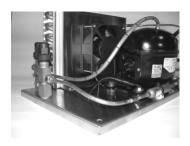
thread the flare nut onto the base valve hand tight. Adjust the bends in the 1/4" copper tubing between the base valve and the filter-drier. When finished, the tubing should route as shown in the photo above.
