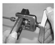
17. Skip this step if a <u>010-1171 compressor</u> was supplied with the kit. Remove the cap on the compressor suction tube nearest the end with the electrical contacts. Use a hammer and the 1/4" swaging tool (079-0661) to enlarge the tube to 1/4", the size of the copper tubing that will be soldered to it.
