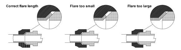
7. Immediately before attaching the flare to the component, apply a small amount of "Leak-Lock" sealant (the blue tube provided in the installation kit) to both sides of the flare. The sealant on the face of the flare will help ensure a leak free connection while that between the back side of the flare and the flare nut itself acts as a lubricant to prevent galling and twisting of the soft copper as the nut is tightened.
