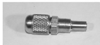
32. Clean the compressor connection tube with the round wire tube/fitting brush (079-2001) as in Steps 12 and 18. Clean the shoulder of the compressor connection tube with the abrasive cleaning pad (079-2010). Insert the cut Schrader valve service port from Step 31 into the compressor connection tube and solder according to preparations procedures mentioned previously in the Preparation Section.
