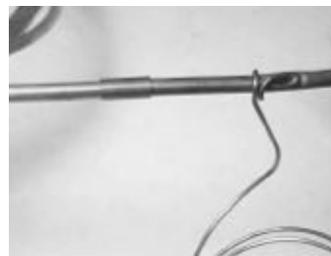
3. Once the 1/4" suction line from Step 2 has been soldered, coil the capillary tube from the evaporator (019-0150) tightly around the 1/4" suction line as shown to the right. The spacing is not critical as this is being done to support the capillary tube and take advantage of any heat exchange between the warm discharge line and the cool suction return line. Coil the capillary tube around the 1/4" suction line until there is only approximately 3" of the capillary tube left.
