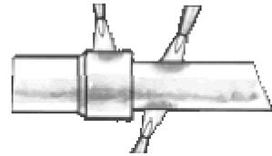
Sweep the flame back and forth along the axis of assembled joint...tubing and fitting...to achieve uniform heat in both parts. Avoid overheating the copper tubing. If the tubing starts turning a dark color and/or begins smoking, it is best to let it cool, re-clean and re-flux the fittings before re-soldering. After the joint is soldered, with the tubing still warm, thoroughly clean the joint of all excess flux using a water moistened rag.
