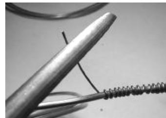
5. After the V notch has been filed into the capillary tube take a pair of pliers and bend the end of the capillary tube at the notch so the end of the capillary tube breaks off. Assure that the end of the tube is open to allow the refrigerant to flow through to the evaporator. The inside diameter of the capillary tube is very small (.022 inch).
