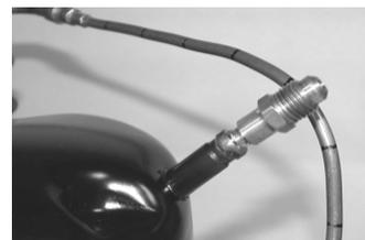
33. After the connection has cooled, install the Schrader valve core from Step 31 back into place, and screw the cap on the valve.
