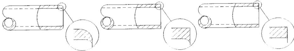
**The proper de-burred tubing should resemble the diagram on the right (pictured above).**
