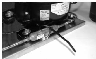
30. **Skip this step if a 010-1171 compressor was supplied with the kit.** Remove the cap on the remaining compressor suction tube. Use a hammer and the 1/4" swaging tool (079-0661) to enlarge this connection tube to 1/4" as in Step 17. Align the swaging tool carefully and strike firmly and squarely with the hammer several times until the swage tool bottoms out against the shoulder of the tube. Remove the swage tool from the tube.
