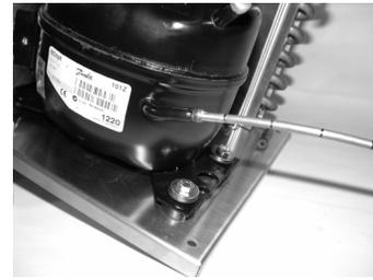
14. Rest the base plate (055-0104) flat after soldering. When the solder joint on the compressor (010-1170) has cooled, gently bend the discharge copper tubing up vertically, and then bend it horizontally towards the top connection tube of the condenser (012-1001). Make large diameter bends and avoid kinking the tubing. Route the tubing within the footprint of the base plate (055-0104).
