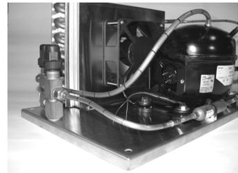
26. Bend the other 1/4" copper tubing end attached to the filter-drier around the other side of the compressor base so that the end will fit into the bottom connection tube on the condenser (012-1001). Bend the tubing carefully to clear the base of the compressor without contacting it. Adjust the bend until the tubing lines up with the lower condenser connection tube, and will insert about 1/4" into this tube.
