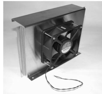
5. Place the fan shroud (055-0181) over the condenser (012-1001). The circular opening of the fan shroud should be on the compressor side with the top of the shroud slipping over the top of the condenser. Line up the two holes in the bottom mounting flange of the fan shroud with the two holes in the base plate (055-0104) and attach with two 1/2" Phillips Pan head machine screws (400-0300) and two Nylock nuts (400-0111). This will capture the condenser and hold it firmly in place.
