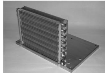
2. Remove the condenser (012-1001) and drill 5/32" diameter mounting holes in the side brackets to match up with the mounting tab holes of the base plate (055-0104).
