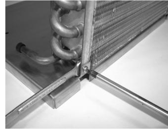
4. Mount the 12vdc condenser fan (071-0125) onto the fan shroud (055-0181) using four 1 3/8" Phillips Pan head machine screws (400-0305) and four Nylock nuts (400-0111). Check the airflow direction arrows on the side of the fan and install it so that the air is pulled through the condenser and discharged out over the compressor. The wires for the fan should be in the lower left hand corner as shown.
