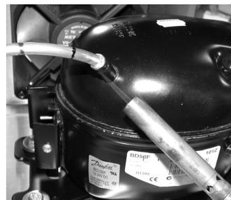
20. After the solder connection has cooled, gently bend the attached 1/4" copper tubing to route it in place to mate it with the male flare fitting on the suction base valve (096-0040) as shown in the photo. Make large diameter bends and avoid kinking the tubing. Tighten the flare nut firmly to the suction base valve with two wrenches.
