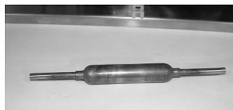
23. Cut a piece of 1/4" copper tubing (025-0032) 7" long, de-burr and clean both ends. Place a 1/4" flare nut (027-0001) over one of the ends and flare the end using preparation procedures mentioned previously in the Preparation Section. Flux the other end and insert into the 1/4" copper union on one of the ends of the filter-drier (020-0500). If there is an arrow on the filter-drier, it should point to the end that has the flare nut. Solder the copper union to the tubing and the filter-drier.
