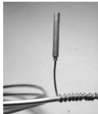
wire tube/fitting brush (079-2001). Insert the cleaned and fluxed 1/4" tubing into the strainer and solder according to preparation procedures mentioned previously in the Preparation Section. Wrap a wet rag over the end of the strainer that has the capillary tube soldered to it to prevent it from overheating. Avoid using too much solder. Label the end of this piece of 1/4" tubing "D", for discharge line, as it will need identification later.
