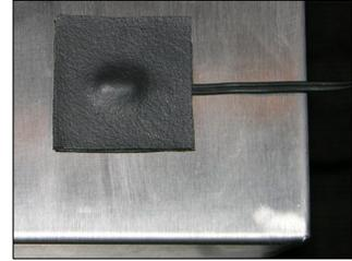
6. Attach the third piece of foam in the same manner as the second piece. Press the layers of foam tape together firmly to assure good contact between the layers.
