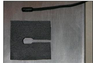
2. Clean the area on the surface of the plate where the probe is to attach. Use soap and water or a suitable solvent such as rubbing alcohol or acetone. The plate surface must be clean, warm, and dry for the insulation tape to adhere well.
