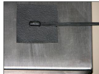
5. Remove the backing from another piece of foam insulation and attach over the probe on top of the first piece of insulation.
