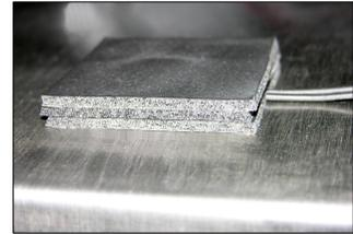
The same foam tape method of probe attachment can be used on the roll bond evaporator. Mount the thermostat probe on a large flat area away from the evaporator tubes and near the exit of the suction line on the roll bond evaporator.
